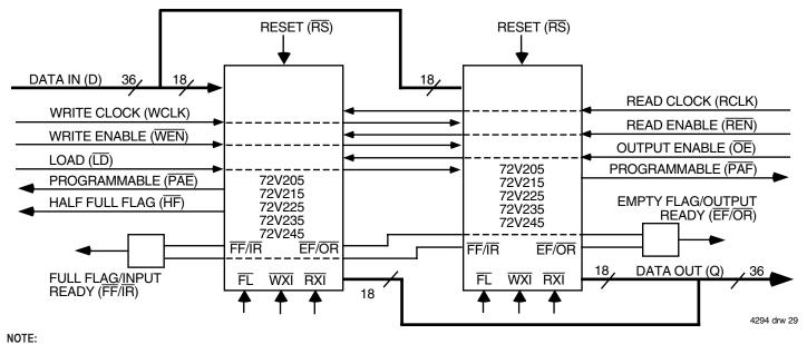
1. Do not connect any output control signals directly together.
