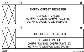
1. Any bits of the offset register not being programmed should be set to zero.
