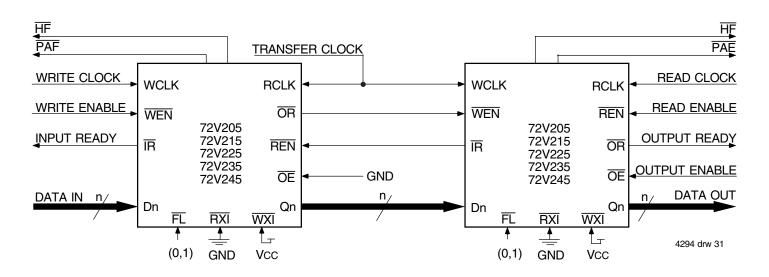
Figure 31. Block Diagram of 512 x 18, 1,024 x 18, 2,048 x 18, 4,096 x 18, 8,192 x 18 Synchronous FIFO Memory With Programmable Flags used in Depth Expansion Configuration
