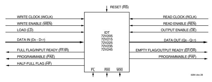
Figure 28. Block Diagram of Single 256 x 18, 512 x 18, 1,024 x 18, 2,048 x 18, 4,096 x 18 Synchronous FIFO
