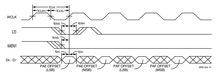
Figure 12. Write Offset Registers Timing
