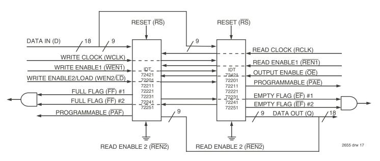
Figure 15. Block Diagram of 64 x 18, 256 x 18, 512 x 18, 1,024 x 18, 2,048 x 18, 4,096 x 18, 8,192 x 18 Synchronous FIFO Used in a Width Expansion Configuration
