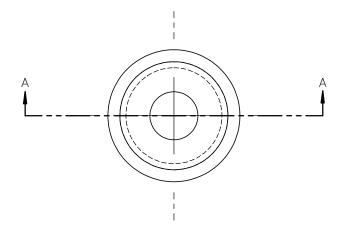
For use with panels of: Max Thickness = 0.063" Hole Dia. = 0.250"
